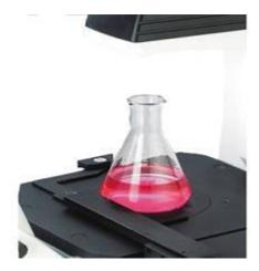
The lab inverted fluorescence microscope has a oversize mechanical stage and a attachment mechanical stage. The moving range of attachment stage is 128mm x80mm, it is available for 96 holes plate. The detachable condenser has a long working distance, for example, this microscope's working distance can reach 195mm when the condenser is detached.
